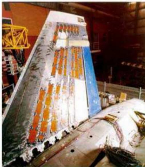
Figure 1. An example of direct-active system: F-18 Fighter instrumented fin with piezoelectric actuators for buffeting control. From Nitzsche et al. (2001).
